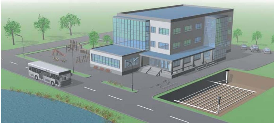
Figure 3: ETAHE with several parallel pipes (Source: Rehau)
